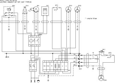
Pressure switch Fan of compressor SP EV1 ST1 Thermo switch EV3 Fan of dryer M1 Motor of compressor FA1 YV1 Breaker Solenoid valve Contactor Terminal KM1 X1 PH1\* Hour counter XC1 Connector Q HL1 Switch Glowlamp Thermo switch of box Fan of box Capacitor ST2 EV4 CB1
