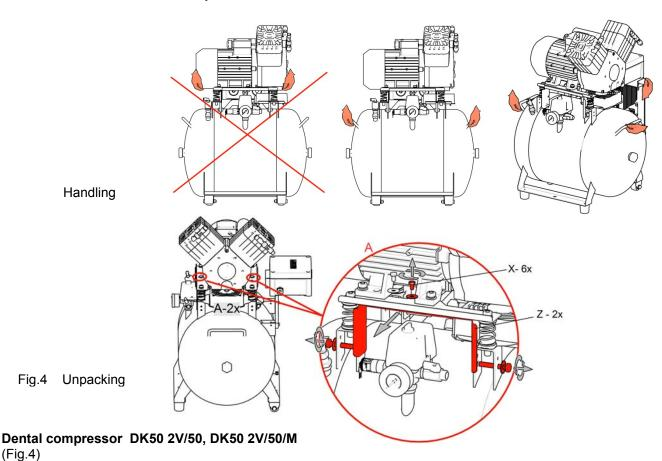
After removing all packaging material, place the product on the floor and remove stabilization parts Y (Detail A). Connect output hose with end-piece to the appliance. Plug the mains cord plug into a socket.
