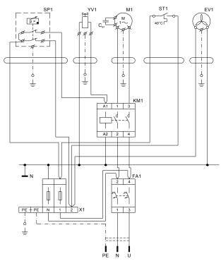
SP1 Pressure switch EV1 Fan of compressor Thermo switch ST1 Motor of compressor M1 FA1 Breaker YV1 Solenoid valve KM1 Contactor X1 Terminal
