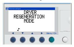
Dryer regeneration for 10 minutes is automatically switched on after 24 hours of compressor operation.
