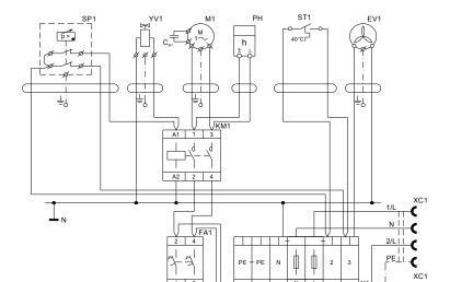
SP1 Pressure switch EV1 Fan of compressor ST1 Thermo switch Motor of compressor M1 FA1 Breaker YV1 Solenoid valve KM1 Contactor X1 Terminal PΗ Hour meter
