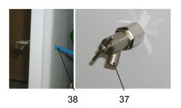
A screwdriver must be used to disconnect the cabinet connector if the compressor is being disassembled! (Fig.6)
