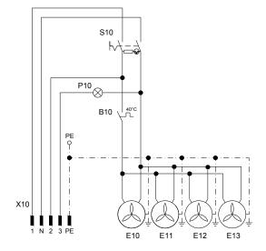
M1,M2 Motor of compressor Q11,Q12 Contactor FA1,FA2 Breaker B2 Thermo switch B1,B3 Pressure switch E1 - E4 E5 – E8 M12 Fan of compressor Fan of cooler Solenoid valve Solenoid valve of dryer M10,M11 K1 X1 B4 Control unit Terminal with fuse Reed switch F3 Fuse E10-E13 Fan of box Connector X2 X10 S10 Switch P10 LED-SERVIS for NDL Cabinet temperature switch
