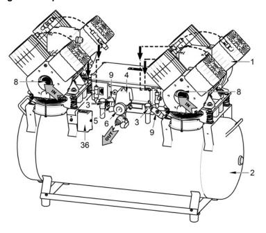
Fig.2- Compressor with membrane dryer (MD)
